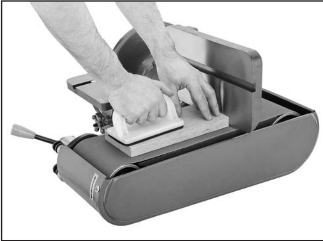
Figure 37. Sanding workpiece in horizontal position.
